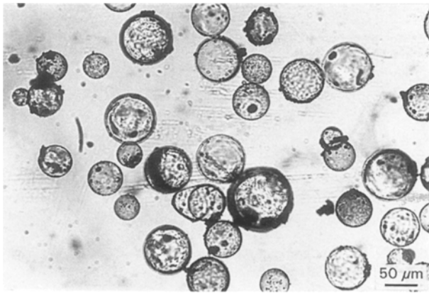
Figure 3 Photomicrograph of cenosphere fly ash.
